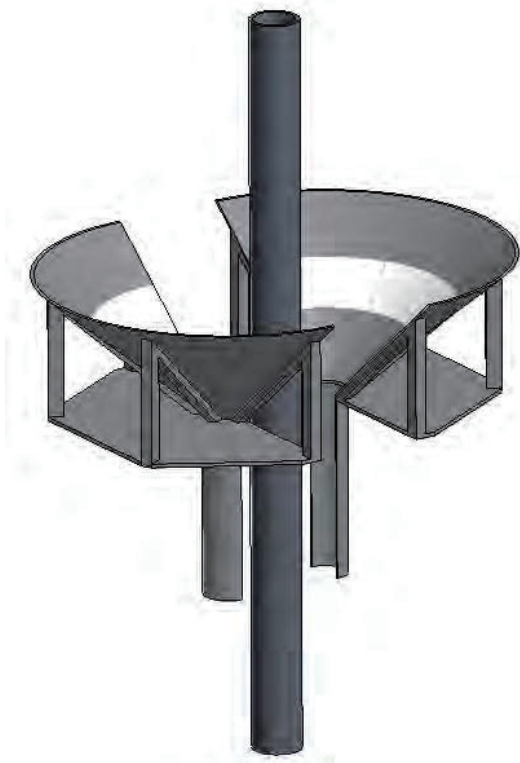
图 4 自由落体重入锥结构 [7] Fig.4 Structure of free-fall funnel [7]
