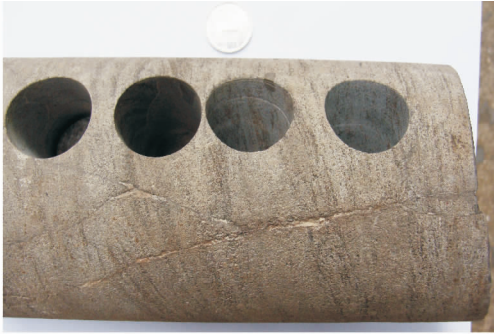
树枝状裂缝(X2井,1 556.5 m,2.5×)
