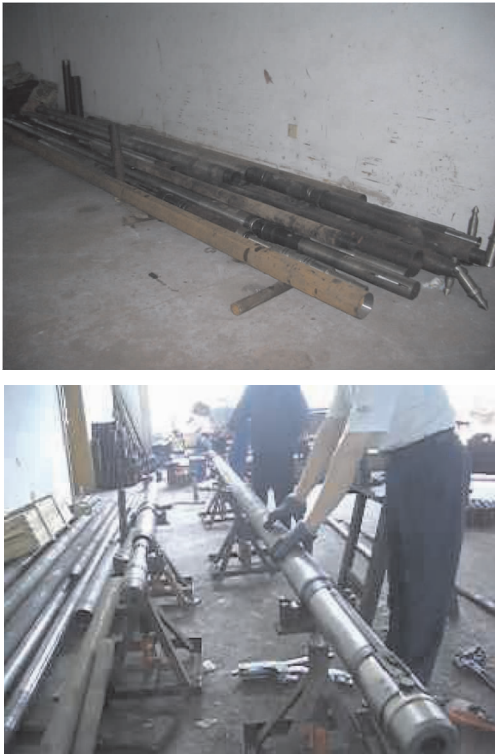
图 2 试制出的保压、非保压取心钻具与室内调试 Fig. 2 Trial-produced pressurized, non-pressurized coring boring tool and indoor debugging
