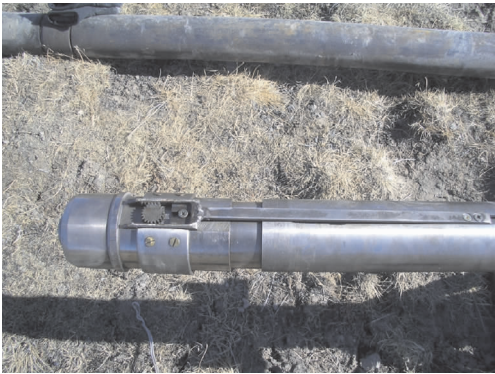
图 3 现场准备下井的保压取心钻具内管一部分 Fig. 3 On-site preparation of part of inner pipe assembly of pressurized coring boring tool for running back into the hole
